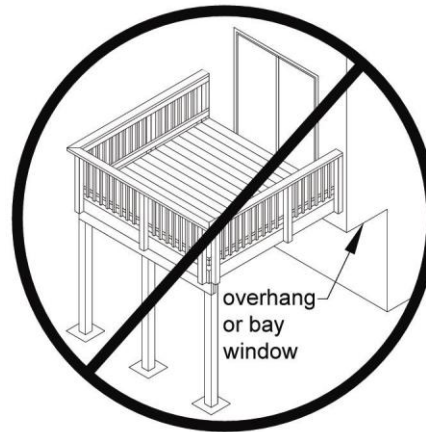
Figure 18. No Attachment to House Overhang with Ledger.
