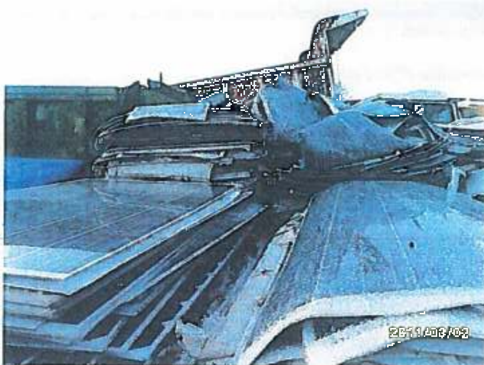
Figure 4: The tangled PV panels in this picture illustrate the nature of broken solar panels, the glass cracks but the panel is still in one piece. Image Source: http://img.cdn.solar.com/p/ma/118259576/broken_solar_panel.jpg
