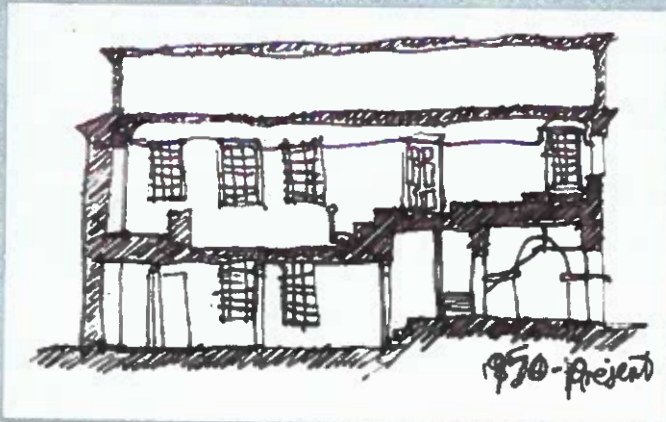
Transverse section (looking toward the North) shows the intermediate floor inserted in 1874-1876.
